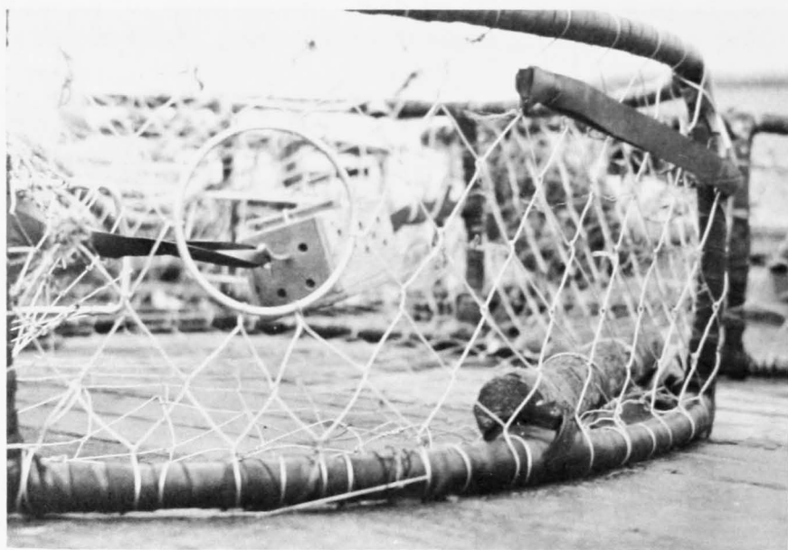
Figure 10.—An escape hatch, one each side allows escapement of female and undersized crabs.
